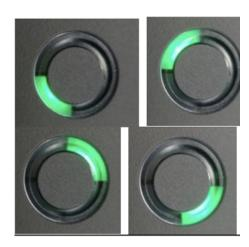
**Solution:** Charge the battery with the charger for at least 30 minutes to ensure the battery's power level is enough. Update the battery with DJI Assistant 2. After the update, mount the battery to the aircraft and check whether there is a warning shown in the app.
